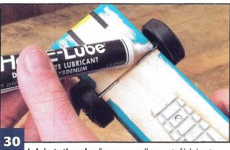
**Lubricate the axles.** Squeeze a small amount of lubricant onto each axle. Use your finger to spin each wheel several times to work the lubricant into the axles. Your car is ready to race!
