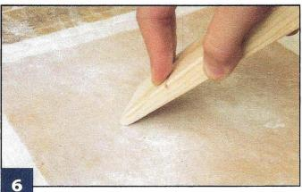
**Sand the edges.** Round the nose of the car. The front of the car should have a smooth taper, rounded from the bottom edge to the top of the car. Unstick the sandpaper and lightly sand the entire car to remove any sharp edges.
