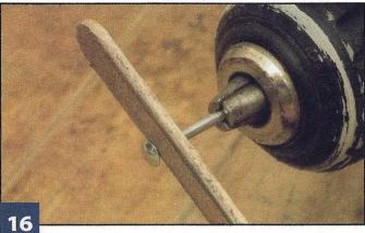
Remove the burrs on the head of the axle. Rotate the sanding stick to remove the burrs under the axle head. Repeat Steps 15 and 16 for the remaining three axles, leaving the last axle in the drill for the next step.
