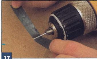
Polish the axle. Cut a sheet of 400-grit wet/dry sandpaper into four ½"-wide strips, each 4" long. Dip the sandpaper into water. With the drill running at medium speed, sand the axle to remove the scratches from the sanding sticks. Keep the sandpaper wet during the entire process.
