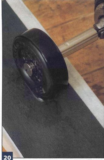
**Remove the mold marks.** Wet the sandpaper. Run the drill at a low speed. Apply only light pressure and sand until the wheel surface is flat and smooth. Repeat for the remaining three wheels.
