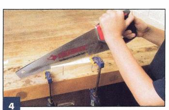
**Cut the car.** Clamp the block to a work surface. Using a hand saw, carefully cut along the line. When you're about halfway through the block, flip it over and cut from the other side.
