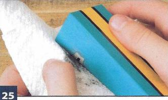
**Lubricate the wheel wells.** Squeeze a small amount of dry graphite lubricant onto a paper towel. Rub the graphite over the wheel slots where the axles attach on both sides of the car. This helps reduce friction where the wheels rub against the car.
