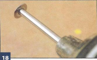
Finish polishing the axles. Rotate the sandpaper to sand under the head of the axle. Change sandpaper strips for each axle and remember to keep the sandpaper wet. Repeat Steps 17 and 18 for all of the axles.
